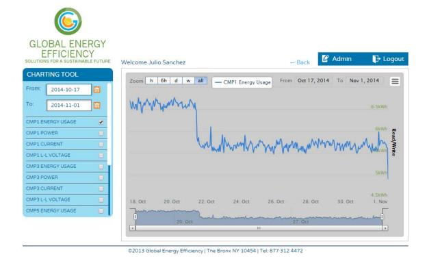
Above are the energy usage plots for CMP1. As the plot shows, before Intellidyne was installed (18Oct-21Oct), the energy consumption was in within the 6.5kWh. The average energy consumption for CMP1 is around 6.6kWh. After Intellidyne was installed (from 22 Oct ), we can notice a significant reduction in the energy consumption. The estimated average energy consumption is around 5.7kWh. This is a **13.6%** energy reduction.
