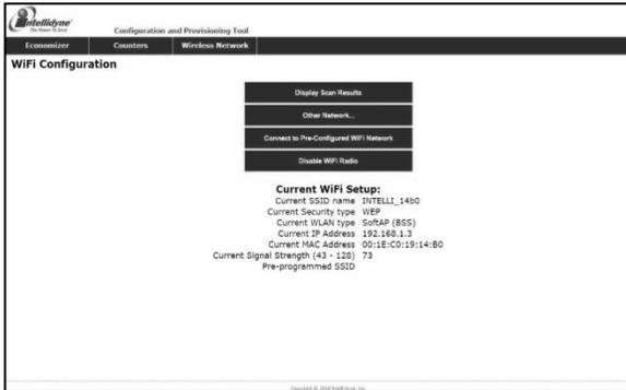
The Wireless Network page is used to view the current Wifi mode of the controller, and to enable the control to join a local network to send its data to a cloud server.
